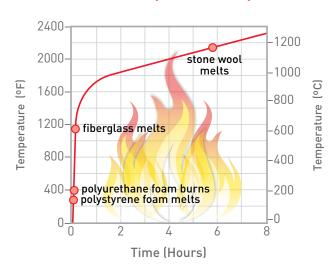
In an application where elevated temperatures are a concern, stone wool will provide greater protection than fiberglass. The maximum service temperature of stone wool insulation when tested to ASTM C411 is 1200 °F (650 °C), compared to fiberglass which is limited to a maximum service temperature of 450 °F (232 °C).
